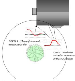
Precise levels confirm movement in the root zone, with maximum of 25mm at the front left hand corner, followed by stations adjoining the bay window.
